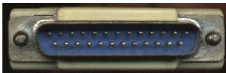
FIGURA 2.6 - FOTO DO CONECTOR DB25 MACHO DO CABO PARALELO.
